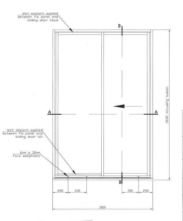
☐ PRELIMINARY ☐ FOR APPROVAL ☐ FOR CONSTRUCTION AS BUILT TITLE 101.6MM COMMERCIAL SLIDING DOOR TEST SPECIMEN DRAFTSMAN BARTOSZ MAZUR TESTING LABORATORY AZUMA DESIGN PROJECT NAME AS2047 COMPLIANCE TEST CHECK DATE C.I 08/08/2016 FORMAT A4 SCALE 1:20
