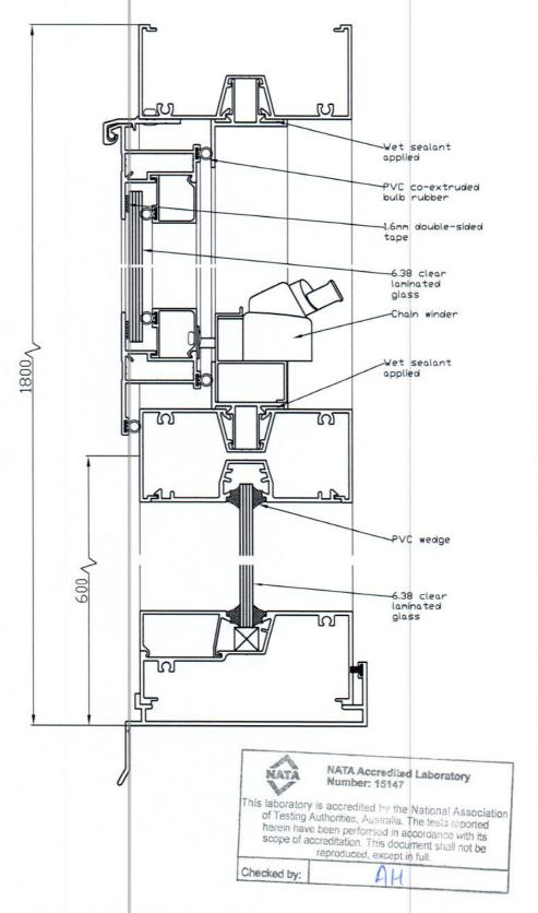
☐ PRELIMINARY FOR APPROVAL ☐ FOR CONSTRUCTION M AS BUILT TITLE COMMERCIAL AWNING WINDOWS TEST SPECIMEN SECTION A-A DRAFTSMAN BARTOSZ MAZUR TESTING LABORATORY AZUMA DESIGN PROJECT NAME AS2047 COMPLIANCE TEST
